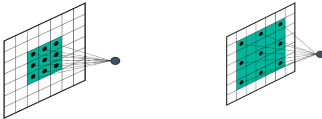
(a) General convolution (kernel 3 \times 3/\text{rate} = 1 ) (b) Dilated convolution (kernel 3 \times 3/\text{rate} = 2 )
